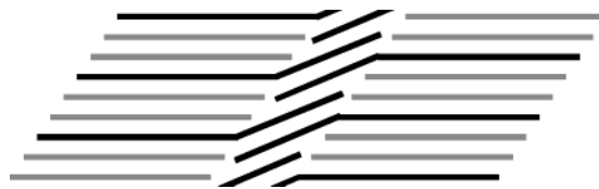
Figure 4. Schematic drawing of the triple-layer superlattice model with the tails in the middle layer adopting a higher tilt angle to counter the deficit of long chains: when the binary mixture contains more short alkane molecules (gray lines) than long ones (black lines).
